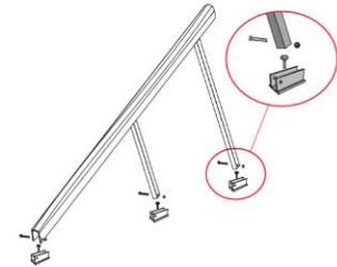
1. • Attach feet to the surface so that they are correctly spaced for the required angle.
