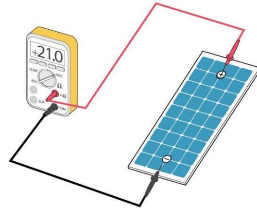
Measuring open circuit voltage or polarity (correct polarity +21 Vdc)
