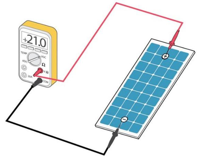
Measuring open circuit voltage or polarity (correct polarity +21 Vdc)
