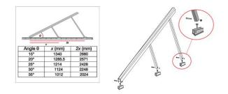
1. • Attach feet to the surface so that they are correctly spaced for the required angle.
