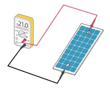
Measuring open cercuit voltage or polarity (correct polarity +21 Vdc)
