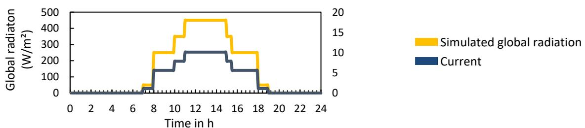
**Figure 1:** Daytime variation of global radiation 3.5 kWh m<sup>-2</sup> d<sup>-1</sup> according to IEC 62124 and exemplary maximum available current during the laboratory test
