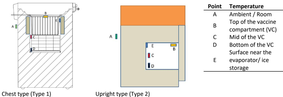
**Figure 3: General position of temperature sensors for the two cabinet types**
